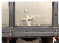
Tests have been successfully performed on offshore platforms and full scale mirrors. But like any other wind tunnel the possibilities are only limited by the test requirements, equipment available and imagination.
