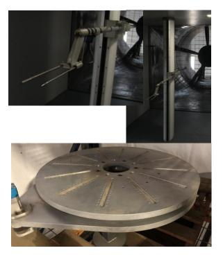
Boundary layer profiles can be accomplished with either spires/ blocks or with a tubing fence.
