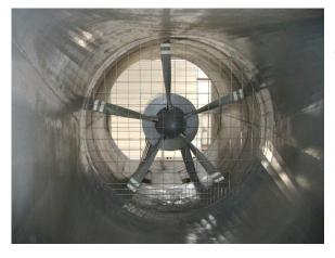
The power section includes 13 ft long diffuser, a 250 hp electric motor operated at a constant RPM (1185), a five (5) blade propeller eight (8 ft) diameter with hydraulic blade pitch actuation to control the wind tunnel wind speed. The facility design includes a long section with constant cross section (32 ft) extending from the nozzle exit to the front of the test section to help with the development of boundary layer profiles.
